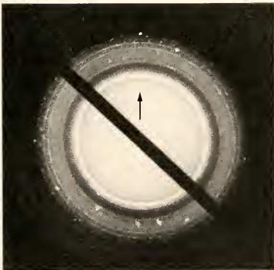
Figure 4. Electron spectroscopic diffraction pattern of the dark region (open circle) in Figure 3 A, showing Debye-Scherrer rings of hydroxyapatite. Black arrow indicates hydroxyapatite {002} lattice planes.
